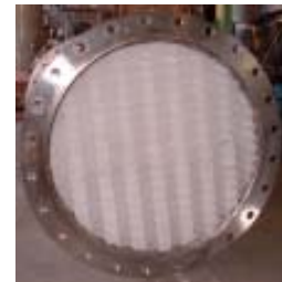
Demister MULTIWIR made of PP mounted in a scrubber
