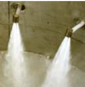
Lances type CSL_DMR with 5 nozzle tips each (quenching system)
