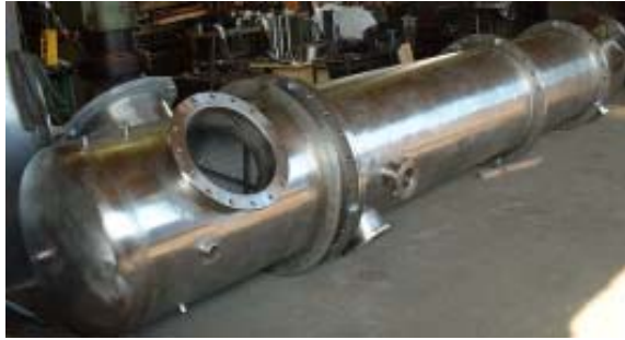
CALWIR scrubber for the separation of boracid aerosols
