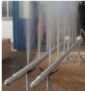
Lances type CSL_DML each with 6 nozzle tips in line (DeNOx-plant)
